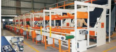
Inspection and packing machines are latest and accurate machines for fabric checking and packing with accurate length measuring device, weighing scale, auto doffer, fabric roll conveying system, damage recording software with display.
