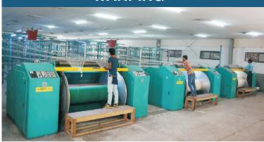
We Have world class warping facilities in separate room with fully computer control and PLC base high speed machine with photo optical stop motions, safety guards, fluff protector, fluff suction and traveler cleaner.
