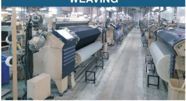
We have Latest Version Picanol (96 Nos.) Tsudakoma (96 Nos.) Air jet Machine with cam and Dobby Shedding motion. We produce various type of weave Combination. i.e. 2/1, 3/1 knitted and Dobby weave denim fabric.
