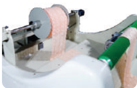
花边机专用置布架 Lace Machine Special Cloth rack
